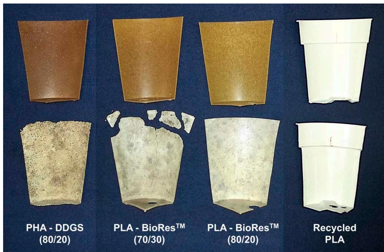
**Figure 1. Samples of one-fourth container pieces as they appeared before (top row) and after (bottom row) six months in garden soil. All four container types were made of very high percentage biorenewable material (99% or more biobased carbon content).**
