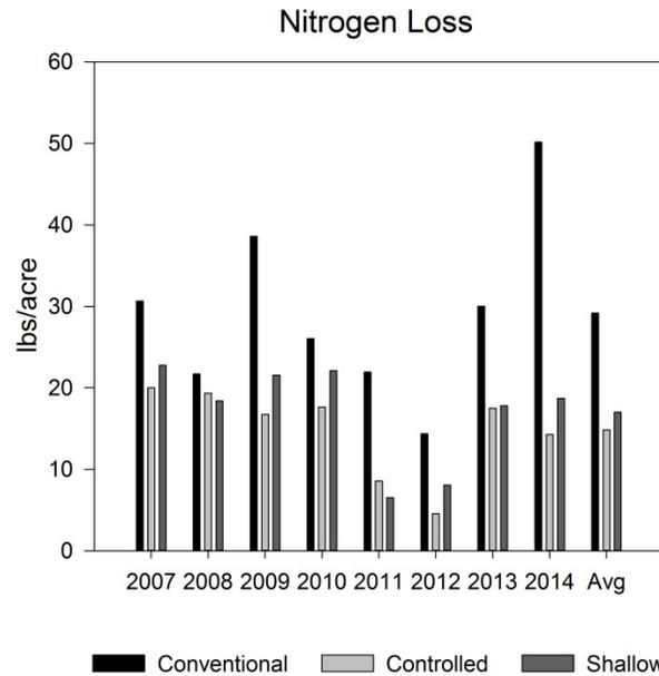
Figure 4. Average yearly nitrogen loss for various tile drainage systems.
